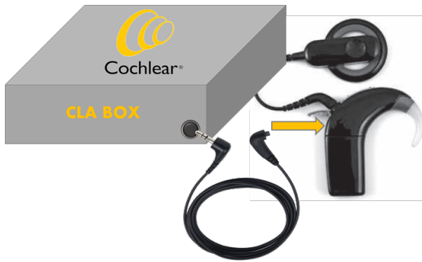
Figure 1: Example of how to connect the CLABOX to the CI via DAI.
