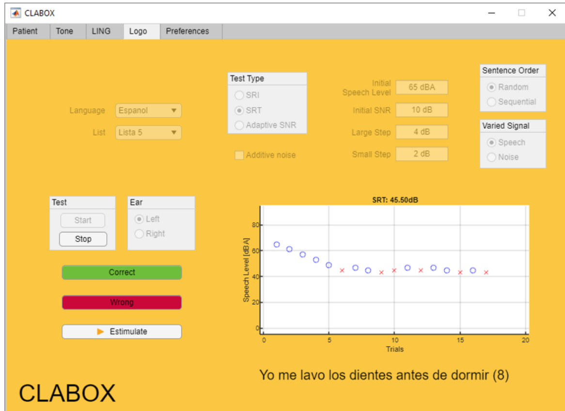
Figure 5: Example of the “Logo” tab, where the examiner can choose between several speech recognition test, adjust their parameters, and test the subject.
