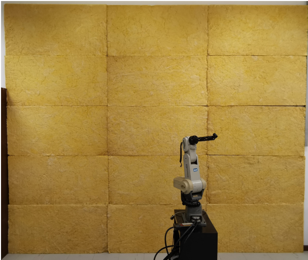
Figure 2: Glass wool absorbing surface and Mitsubishi RV-M1 robotic arm.
